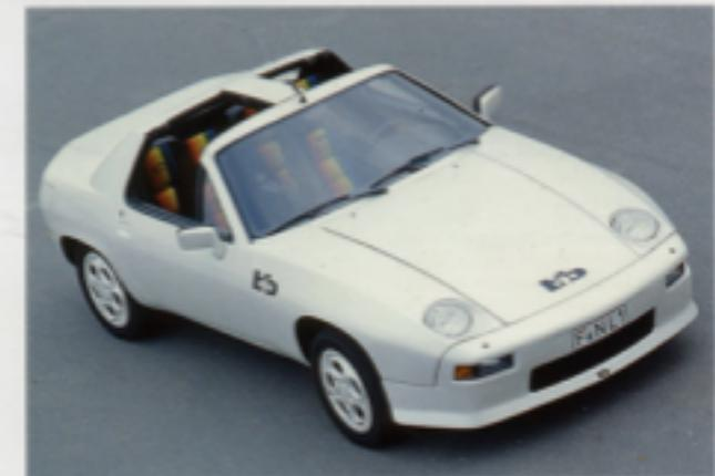
Unlike the standard version with its conventional covered pop-up headlamps, b+bi used the 928 system where the lamp lens remained exposed and the inside of the car was again to a very high standard in sound (16 speakers!) and comfort.
